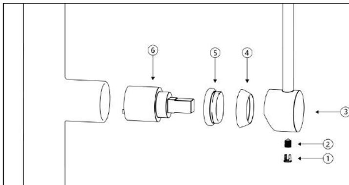
1. Take out the handle cap (1) and use the allen key to screw out the grub screw (2) .
