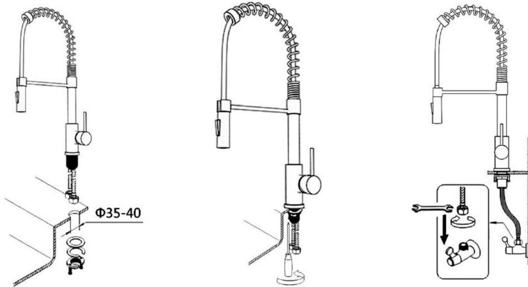
1. Identify all components are present prior to starting installation .
